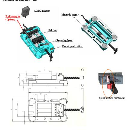
$Feature: \bullet \ \ \text{Magnetic base is designed for prostioning the vise on the working table accuractely \& promptly}$
