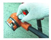
7. Slip the pipe guide at the rear of the threader over the pipe and gently apply pressure to the front end of the die head and moving the handle down at the same time in order to make the dies engage into pipe
